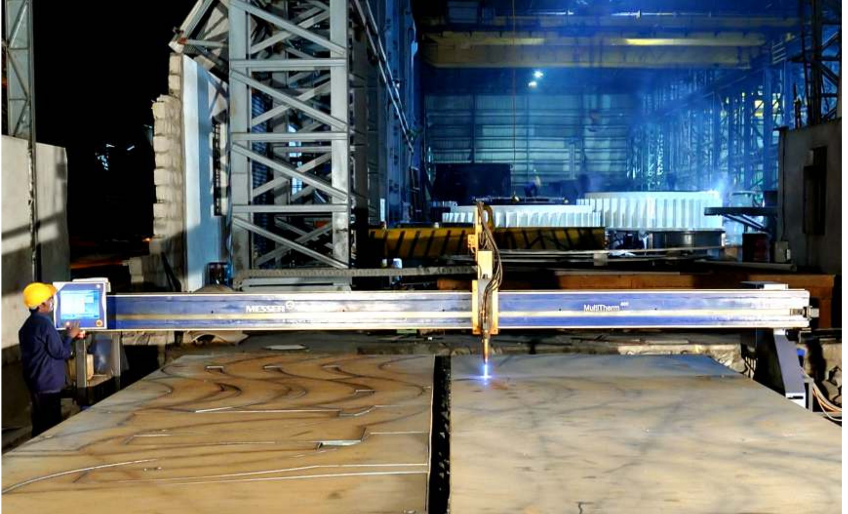
Profile cutting machine with cutting thickness up to 300mm
